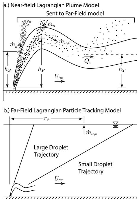
Fig. 7. Schematic of the nearfield plume models and farfield models indicating the locations of the metrics reported in the model intercomparison figures.
