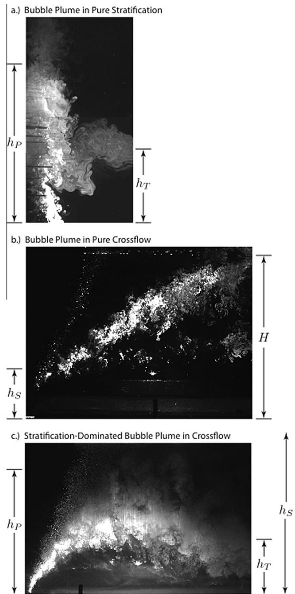
**Fig. 1.** Dye visualization of bubble plumes in laboratory experiments for (a) pure stratification with no crossflow ( $h_s = \infty$ ) (adapted from Seol et al. (2009)), (b) pure crossflow with no stratification ( $h_p = \infty$ ), and (c) combined effects of stratification and crossflow for a stratification-dominated plume ( $h_p < h_s$ ).
